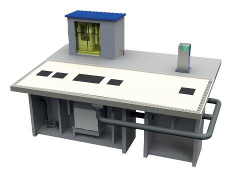
The Facet Car Wash Water Reuse Systems UR Series, have been designed to treat water coming from car washes (manual, automatic, in boxes, washing tunnels...) of personal, industrial and agricultural vehicles, etc.
